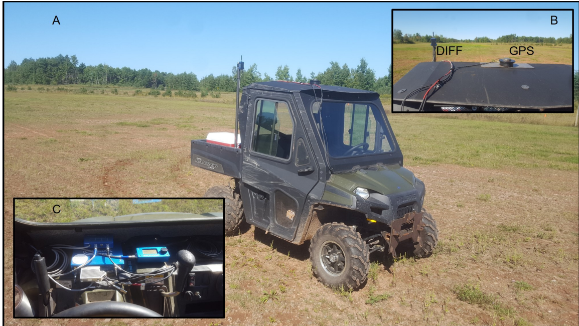
Figure 4.12 (A) Polaris Ranger driven around the test sites at KRC. (B) GPS/GLONASS antenna and differential correction antenna (C) VBOX GPS System in Ranger cabin.
